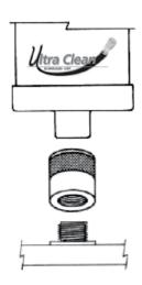
Spin-on Adapter Model UC-AD105 (1" - 12 UNF) Model UC-AD106 (1½" - 16 UN)
