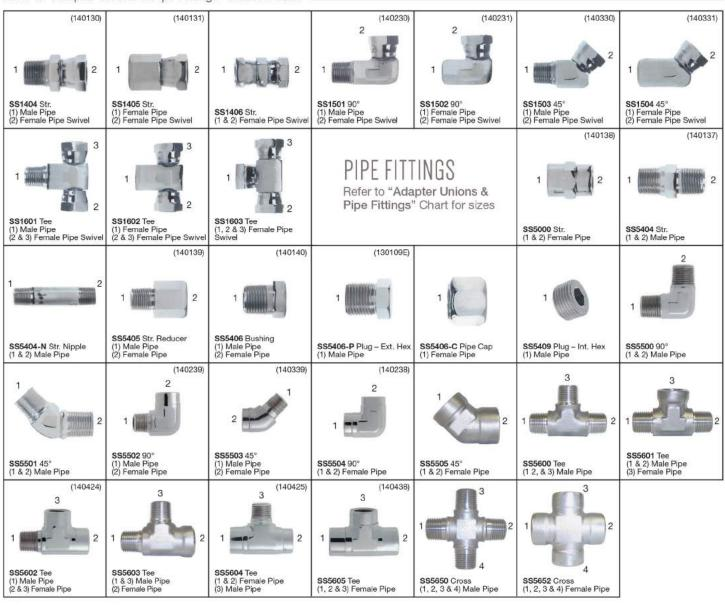
**ORDER INFORMATION** Sizes of the fittings are indicated by the dash numbers as relating to sixteenth's of an inch measured from the Outside Diameter of the tube size used. For example; 1/2" O.D. (8/16) or – 8. Male or Female pipe sizes are similar in that 1/2" pipe thread is also (8/16) or – 8.
